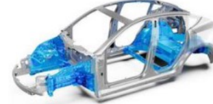
Simplification of vehicle Body in White Structure
