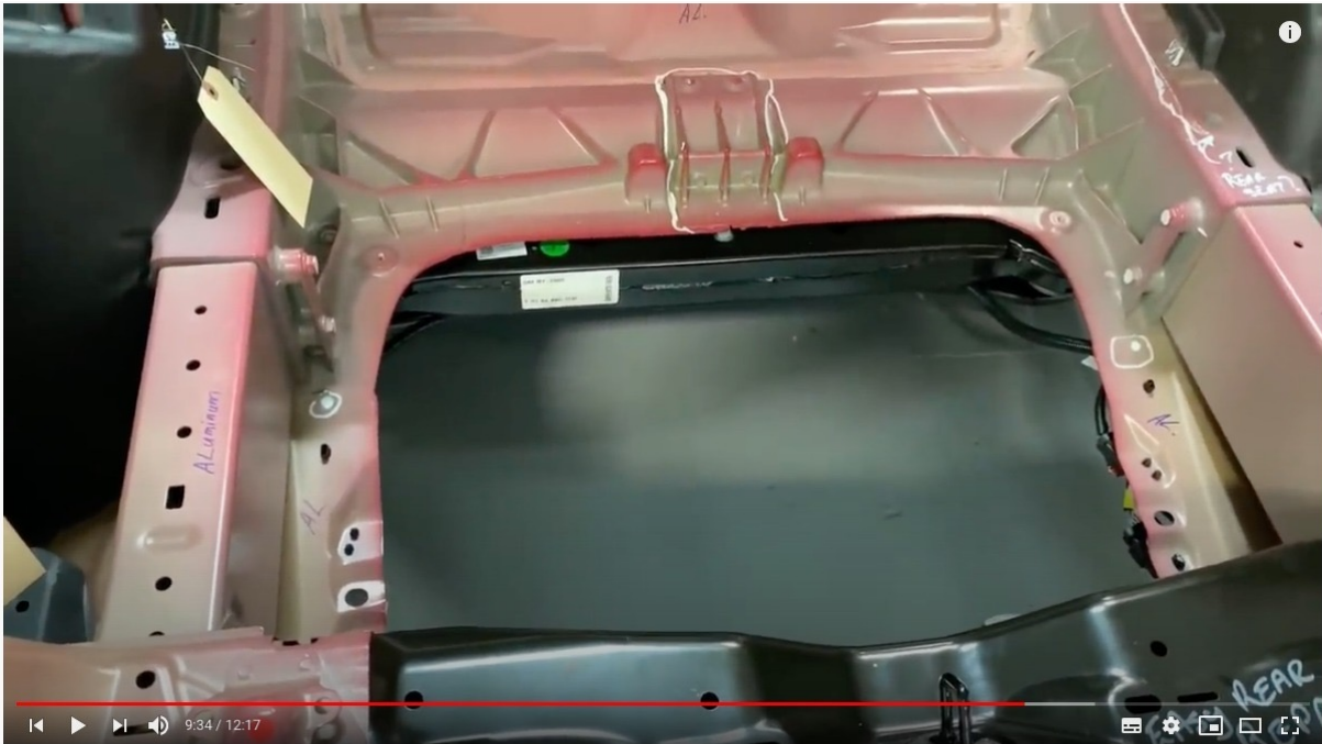
Model Y E14: Rear Mega Castings and Structure, Trunk Tub, Potential Tow Location
